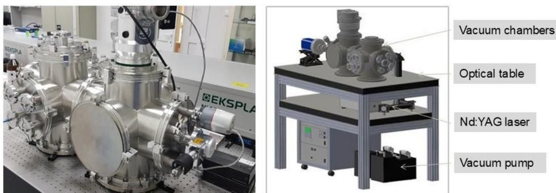
Fig. 1. The view of the XAFS/CT laboratory workstation and its CAD design.
