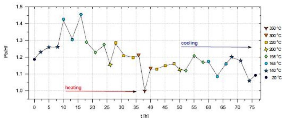
Figure 1. The changes of atomic concentration in the Pb/Hf ratio obtained for the *as grown* PbHfO<sub>3</sub> single crystal in wide range of temperatures obtained from the XPS study.
