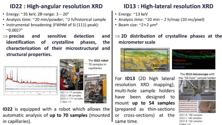
Figure 1. The two X-ray diffraction beamlines accessible through the "historical materials BAG" access: ID22 and ID13
