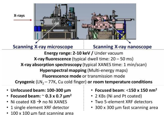
Figure 3. The scanning X-ray microscope and nanoscope at ID21: X-ray absorption spectroscopy at the sub- micrometric scale
